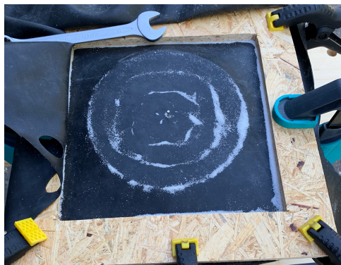
Figure 10: My only successful Chladni figure with the 3D-printed frames
