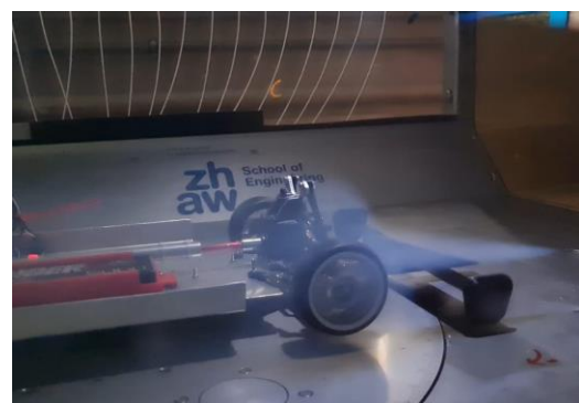
Figure 52: Wheel Spin Influence on Air
